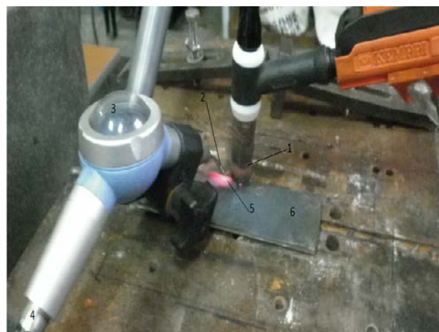
Fig. 5. Insertion of nano-powders behind the weldseam in the low temperature area 1 – nozzle; 2 – insertion tube for nano-powder and inert gas; 3 – nano-powder reservoir; 4 – inlet for the protection gas argon; 5 – heated metal right after the arc goes out; 6 – work piece.
