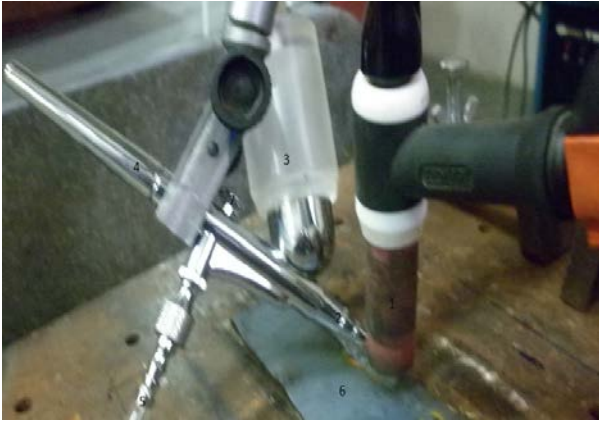
Fig. 6 Insertion of nano-powder behind the arc of welding in the low temperature area.
